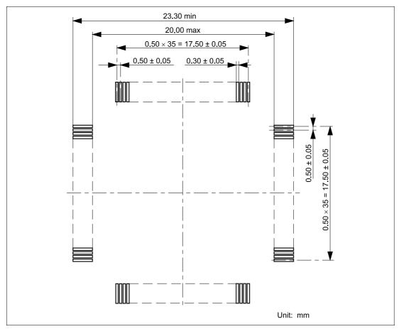
Figure 5 Recommended Dimensions for Mount Pad
